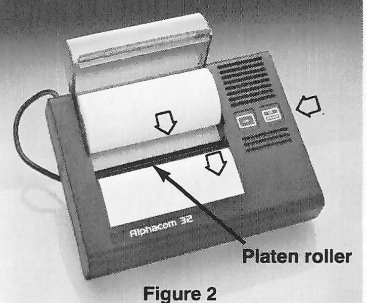
INTRODUCTION The Alphacom 32 printer gives a permanent record of anything your Sinclair ZX81<sup>®</sup>, or Sinclair Spectrum<sup>®</sup> can display on the TV screen.
